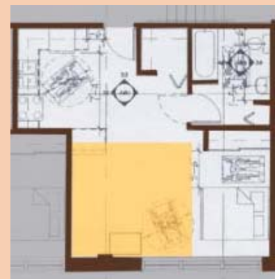
The new floor plan includes jogs in the walls to help create distinct living spaces in each unit. In contrast, the shaded area represents the previous unit's footprint.
